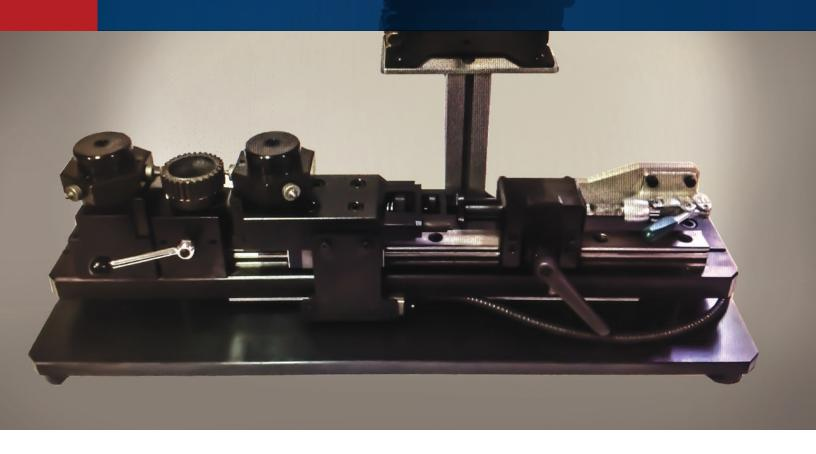
Veit Tool & Gage Dimension over ball/pin DOB/DOP gages are used typically to measure pitch diameters of gears and splines, but not limited too. Our gages are designed for accuracy, durability and ease of use, with consistent upgrades as technology advances. They are very versatile in their ability to accurately measure a variety of part features.
